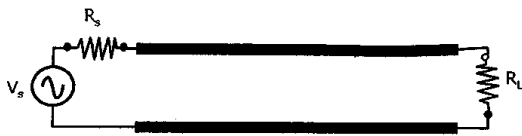
Figure 1a. A finite-length transmission line, the time-domain voltage source, v_s(t) , and the source resistor, R_s , terminated by a complex load, R_L .
